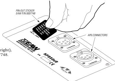
If the input has two AP6 connectors (shown right), cover the pin-out code with sicker P/N 0007748.
