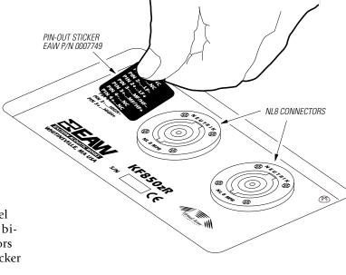
10. The pin-out code on the existing input label must be replaced with a new sticker with the biamp code. If the input has two NL8 connectors (shown above), cover the pin-out code with sticker P/N 0007749.
