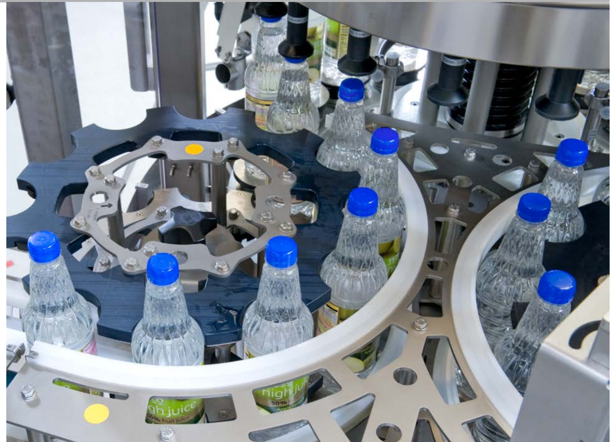
Raptec handling parts at a labeller
