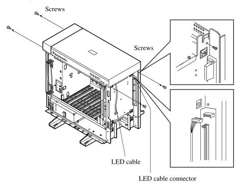
**2.** Remove the top cover by loosening the four screws.
