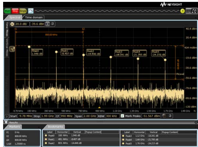
Peak readouts in the FFT plot.
