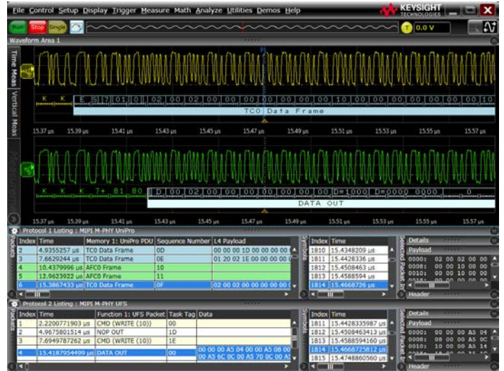
Packet decode and CRC verification through the oscilloscope MIPI UniPro and UFS protocol decoders.
