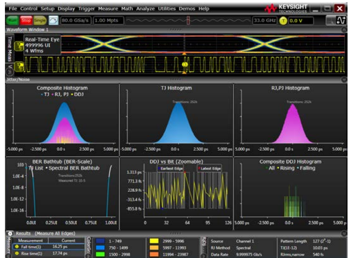
Multiple jitter analysis plots for enhanced visualization.
