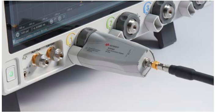
N7010A active termination adapter provides a low noise single-ended cabled measurement solution with 50 \Omega voltage termination ( V_{\text{TERM}} ) up to 30 GHz bandwidth.
