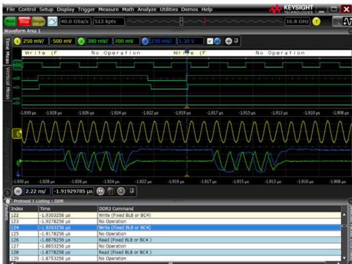
DDR3 protocol decode and write command trigger.
