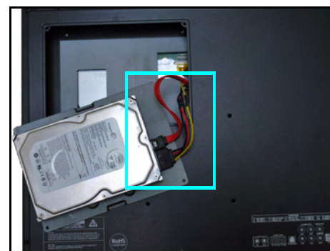
Remove the plate, but be careful not to damage the power and data cables.
