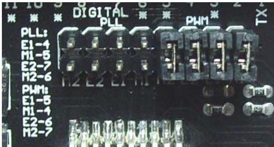
Figure 2 Control Mode Selection Jumpers
