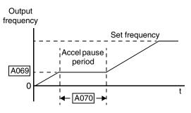
direction while the inverter is in a Stop mode. Initiating a normal acceleration in such a situation may result in over-current trips. This function can be used to keep the inverter output frequency and voltage at low levels long enough to bring the load to a stop, and commence turning in the desired direction before the acceleration ramp resumes. See also <u>"DC Braking Settings" on page 3–17</u>.
