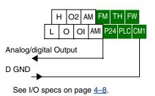
The following table lists the configurations for terminal [FM]. Use function C027 to configure.
