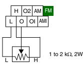
**Voltage Input** – The 0–10V voltage input circuit uses terminals [L] and [O]. Attach the signal cable's shield wire to terminal [L] on the inverter only. DO NOT ground the shield at its other end. Maintain the voltage within specifications (do not apply negative voltage). Normally a full-span input level (10V) will give the maximum motor frequency. You can use parameter A014 to select a lower voltage for full output frequency (such as using a 5V input signal).
