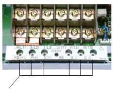
Retention screws locations for capacitor bank
