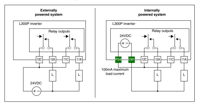
If you use an external supply to power the load(s), the relay contacts can switch up to several amperes. See <u>"Specifications of Control and Logic Connections" on page 4–8</u> for relay contact ratings.
