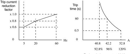
**Constant Torque Characteristic** – The left graph below shows the effect of the constant torque characteristic curve. For example, at 2.5Hz, the output current level to cause overheating in a fixed time period is reduced by a factor of 0.9. The right graph below shows the reduced trip current levels in those conditions for given trip times.
