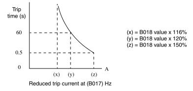
**Thermal Warning Output** – Using parameter C061, you can set the threshold from 0 to 100% of trip level for turning ON the intelligent output [THM] at that level. In this way, the inverter provides an early warning before the electronic thermal overload trips and turns OFF the output to the motor.
