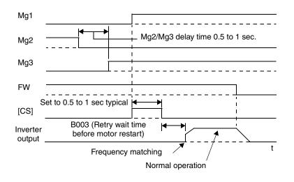
In the previous timing diagram, when the motor has been started across the line, Mg2 is switched OFF and Mg3 is switched ON. With the Forward command to the inverter already ON, the [CS] terminal is switched ON and relay Mg1 contacts close. The inverter will then read the motor RPM (frequency matching). When the [CS] terminal is switched OFF, the inverter applies the *Retry wait time before motor restart* parameter (B003).
