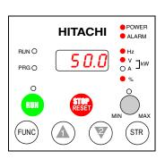
For the powerup test, monitor the motor speed indirectly by viewing the inverter's output frequency. The *output frequency* must not be confused with *base frequency* (50/60 Hz) of the motor, or the *carrier frequency* (switching frequency of the inverter, in the kHz range). The monitoring functions are in the "D" list, located near the top left of the diagram in the <u>"Keypad Navigational Map" on page 2–25</u>.
