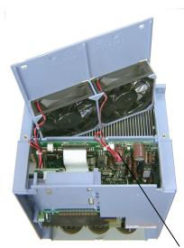
PWB connector for fan assembly wiring
