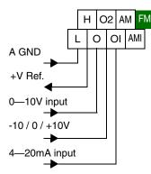
the inverter output frequency. The [AT] terminal function is covered in <u>"Analog Input Current/</u><u>Voltage Select" on page 4–25</u>. Remember that you must also set A001 = 01 to select analog input as the frequency source.
