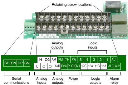
Specifications for the logic connection terminals are in the following table:
