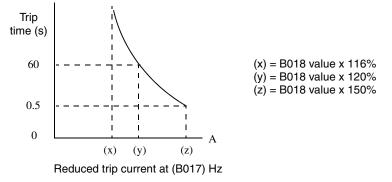
Any intelligent output terminal may be programmed to indicate a thermal warning [THM]. Parameter C061 determines the warning threshold. Please see <u>"Thermal Warning Signal" on page 4–47</u> for more details.
