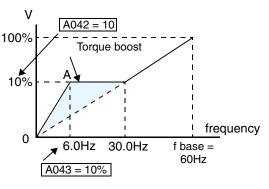
addition to the standard straight V/f line (constant torque curve).
