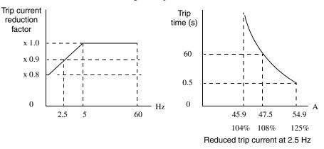
**Free Thermal Characteristic** - It is possible to set the electronic thermal characteristic using a free-form curve defined by three data points, according to the table below.
