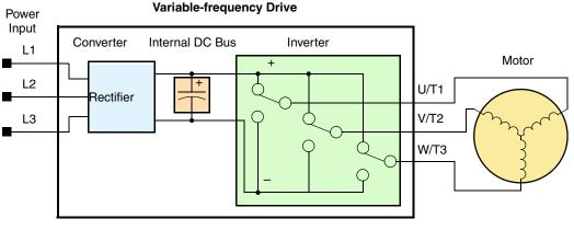
The simplified drawing of the inverter shows three double-throw switches. In Hitachi inverters, the switches are actually IGBTs (isolated gate bipolar transistors). Using a commutation algorithm, the microprocessor in the drive switches the IGBTs ON and OFF at a very high speed to create the desired output waveforms. The inductance of the motor windings helps smooth out the pulses.
