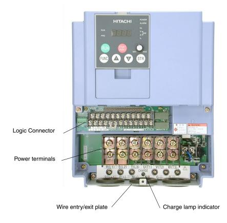
**WARNING:** Be sure to wait five minutes after powerdown and verify the charge lamp indicator is OFF to proceed. Otherwise there is the risk of electric shock.
