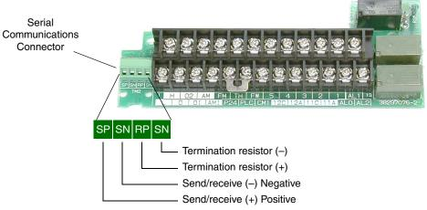
Serial Connection The serial connector is to the left of the control logic connector as shown below: Diagrams
