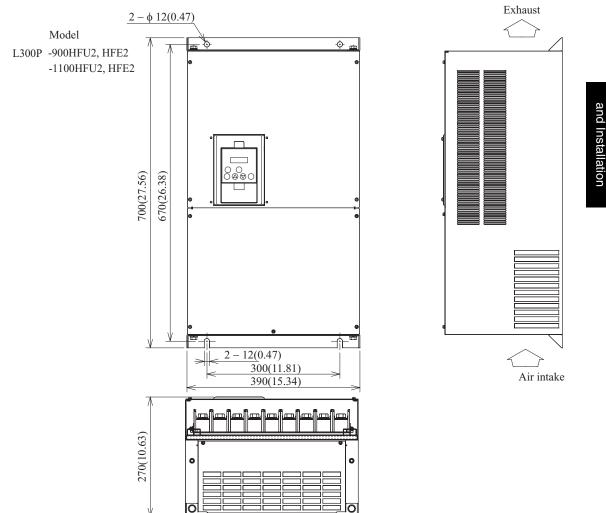
Inverter Mounting and Installation
