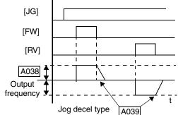
A jog command may arrive while the motor is running. You can program the inverter to either ignore or respond to a jog command in this case by using function A039. The type of deceleration used to end a motor jog
