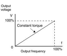
dented accuracy. The L300P utilizes these devices to perform complex mathematical calculations required to achieve superior performance. You can choose various torque curves to fit the needs of your application. Constant torque applies the same torque level across the frequency (speed) range. Variable torque, also called reduced torque, lowers the torque delivered at mid-
