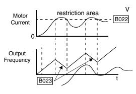
controlled deceleration, the inverter monitors both output current and DC bus voltage. The inverter will increase output frequency to try to avoid a trip due to over-current or over-voltage (due to regeneration).
