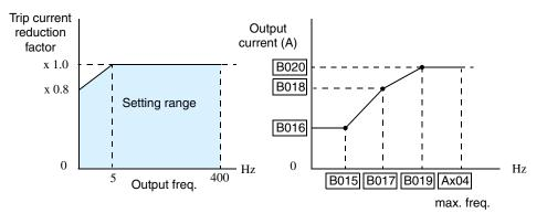
Suppose the electronic thermal setting (B012) is set to 44 Amperes. The left graph below shows the effect of the free setting torque characteristic curve. For example, at (B017) Hz, the output current level to cause overheating in a fixed time period is reduced by a factor of (B018). The right graph below shows the reduced trip current levels in those conditions for given trip times.
