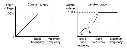
The graph above (right) shows the general characteristic for variable torque. The curve may be best described in three sections, as follows:
