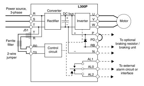
To provide power to the control circuit after input power loss, you must change the control circuit wiring as shown below (steps provided on following page).
