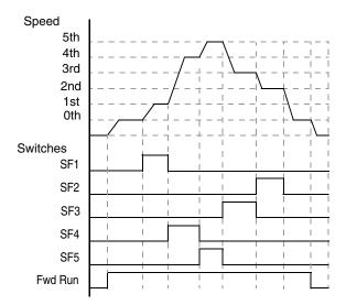
Note: Input functions SF6 and SF7 may be substituted for any of SF1–SF5, to access Speed 7 or Speed 8.
