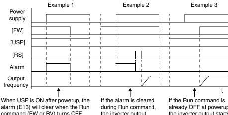
alarm (E13) will clear when the Run command (FW or RV) turns OFF.
