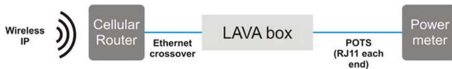
Figure 12: Ether-Serial Link bridging power meter and cellular router
