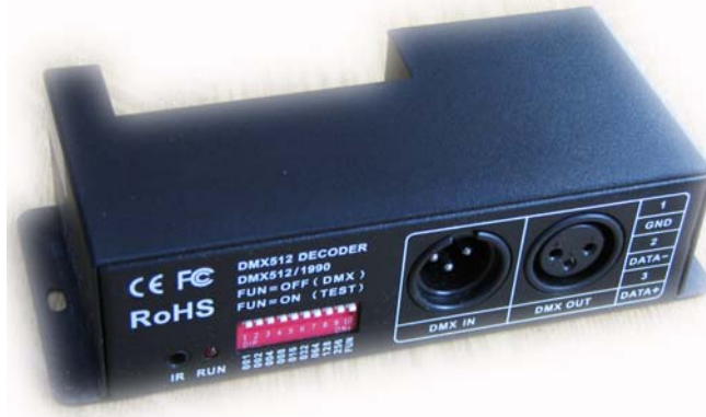
Figure 18: DMX 512 Lighting Control
