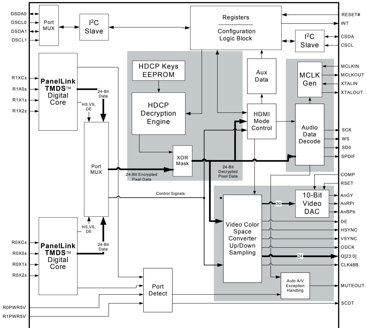
The Sil 9021 supports two HDMI input ports. Only one port may be active at any time.
