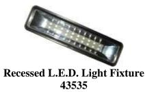
Recessed LED Light Fixture. Available in white 5500K. 12 VDC. Approximate size 2.25 wide, 8.75 length and 1 depth. Uses 300mA @ 13.8 VDC. 4.1 Watts power consumption. Equivalent to a 40 watt light bulb. Has mounting clips to secure from the inside. Has a glass lens.
