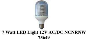
600 Lumen output. Comparable to a 55 Watt Incandescent. 5.8 Watt power consumption. 420 current consumption. Available in white 6000 Kelvin. Long life of 60,000 hours. E27 screw in base. 12V AC or 12V DC. 2.70 inches diameter x 5.93 inches height. 7 Watt LED Light 96 LEDs. This LED Light is not dimmable. Great for desk lamps, landscaping, holidays, everyday lighting, airports, landing strips. UL, C-UL and CE listed. One per package. Uses 450mA @13.8 VDC.
