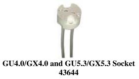
GU4.0, GX4.0, GU5.3 and GX5.3 Socket with pigtail. Use this socket for G4, MR11 and MR16. The wires are 6 inches 18 AWG stranded copper with silicon insulation. The body is ceramic and metal. Rated 250 VAC 12.5 amps.
