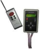
Electronic Digital RF Flexible strip controller 5Volt DC 73532
