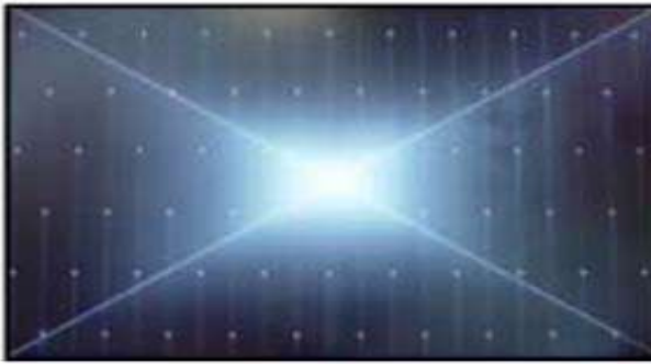
Solder defect, Short/Crack
