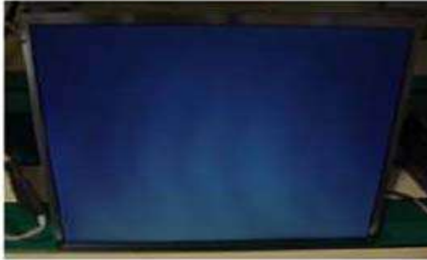
Panel Mura, Light leakage
