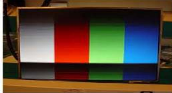
Horizontal Block Gate TAB IC Defect
