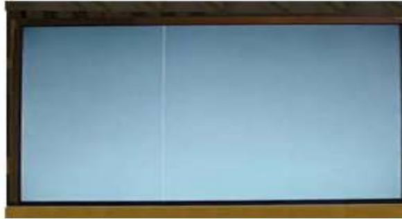
Vertical Line Source TAB IC Defect
