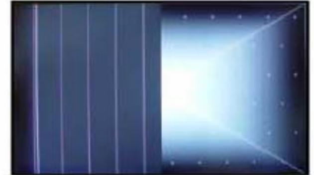
Solder defect, CNT Broken
