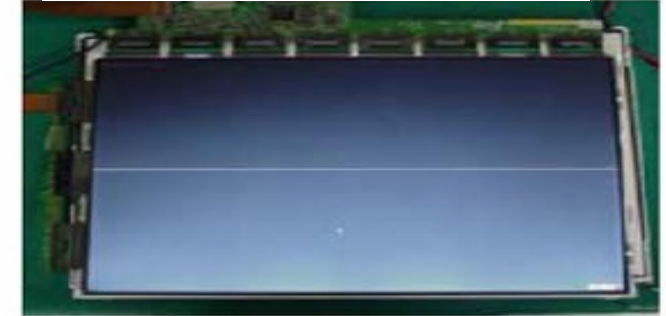
Horizontal line Gate TAB IC Defect
