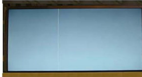
Vertical Line Source TAB IC Defect
