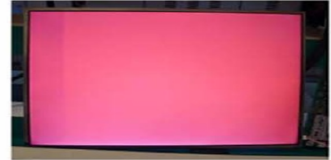
Vertical Block Source TAB IC Defect
