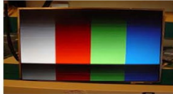
Horizontal Block Gate TAB IC Defect
