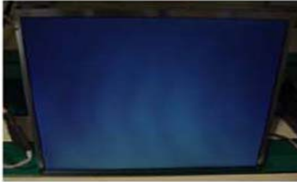
Panel Mura, Light leakage
