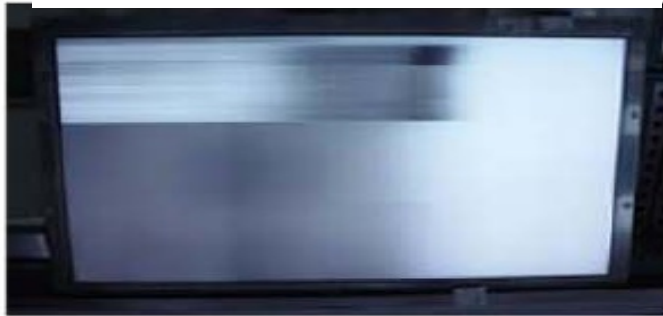
Horizontal Block Gate TAB IC Defect
