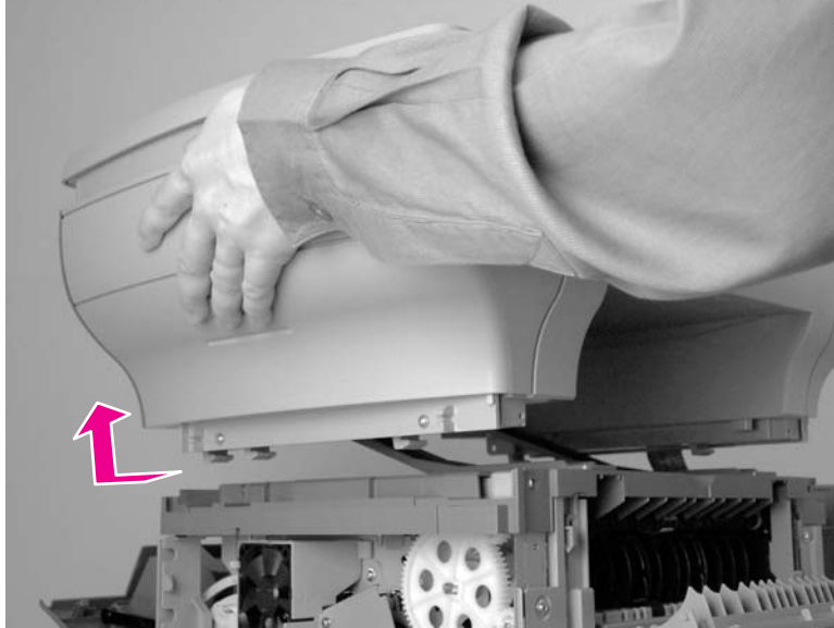
Figure 5-40. Separate the scanner from the printer (4 of 4)
