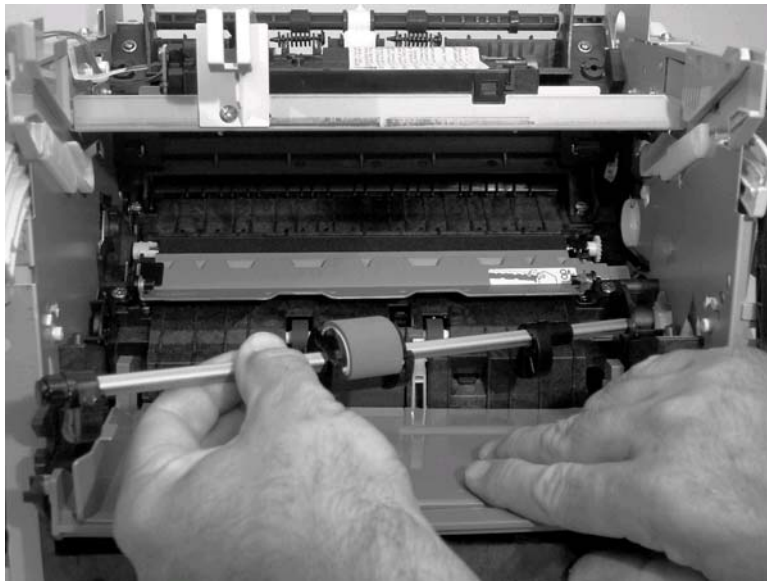
Figure 5-82. Remove the pickup roller shaft
