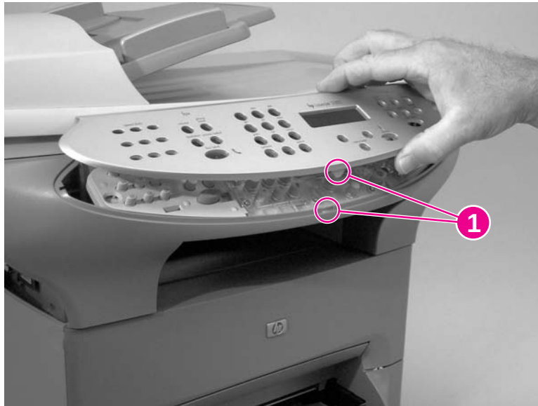
Figure 5-23. Reinstall the control-panel bezel (1 of 2)
