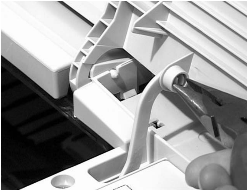
Figure 43. Disconnecting the toner cartridge drive arm
