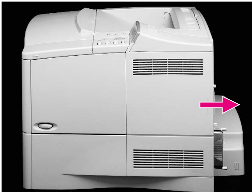
Figure 40. Removing the rear right side cover
