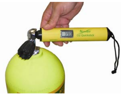
Use Independent Oxygen Analyzer for Verification
