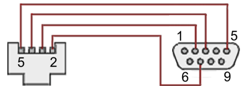
RJ11-to-DB9 RS232 cable with rear view of DB9 connector to PC
