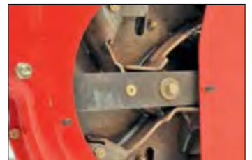
Specially hardened self cleaning steel blades
