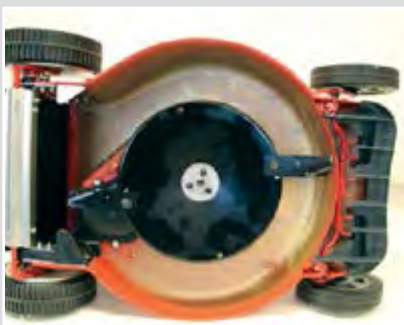
Cutting disc accepts 2 or 4 swing back blades to give crankshaft protection
