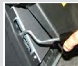
Single 6 position lever that adjusts the mower evenly from 15mm to 65mm.
