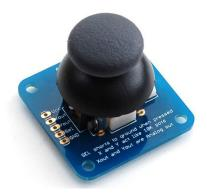
To be able to interact with the kit, we have a tiny joystick. Apart from moving it back and forth, up and down, you can also press it down as a button
