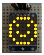
Here we have a <u>LED matrix</u>. Basically 64 LED lights in 8 rows of 8. It is mounted on a small board that has a chip that makes it easier to control
