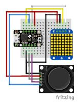
The image to the left shows how the signals between the three hardware components are connected. All you need to build this kit is a small soldering iron and some wires. And of course some basic electronics building skills. If you come to the IKEA maker space at IKEA 2, we'll help you with all that!
