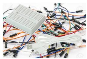
The rest are what we call "electromechanics": A plastic prototyping platform called "<u>breadboard</u>", a USB cable to connect to the PC and small wires
