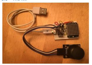
This is what the kit looks like when it is all connected. It fits in the palm of your hand. The two main features, are the LED matrix the tiny joystick.
