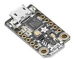
This is the <u>microcontrolle</u>r, the "brain" of the system. It has a USB connector to connect to our PC and sockets to connect the other components
