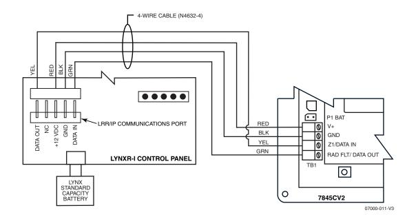
2. The diagram that appears on the bottom of page 9 of the LYNXR-I Installation and Setup Guide reversed the colors of wires at where they are connected to the AlarmNet 7845i-ENT/7845i.
