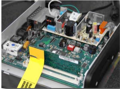
Figure 3-53 SIMM Battery Strip
