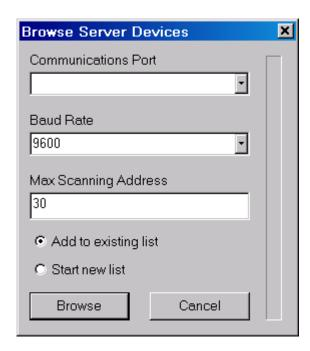
Select the communications port which is connected to the Omega Engineering instrument and the communications baud rate. You may also specify the highest ModBus address to scan for devices on, this defaults to 30 but can be set as 1 to 254.
