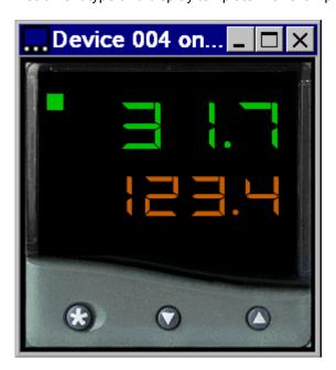
Note: the instrument display will show LEV5 if no valid setting has been made for input sensor, display resolution or output device, these settings are configurable from instrument front panel only.
