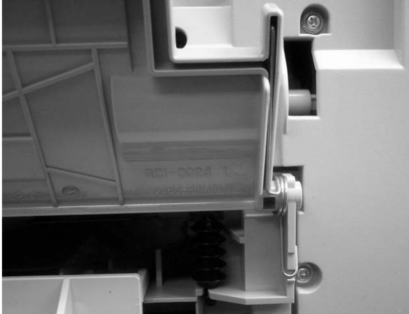
Figure 5-79 Correct tray 1 rear-hinge-spring placement
