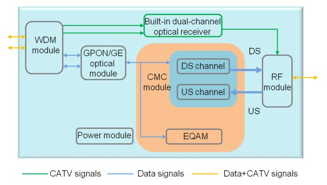
Functional modules include the power module, optical receiver/transceiver module, CMC module, and RF module, which are separate modules and can be replaced onsite.
