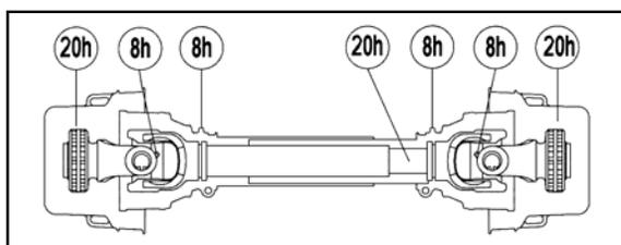
Every 20 hours slide the PTO shaft apart, clean the telescopic tubes with kerosene and apply multi-purpose grease to the sliding surfaces, then reassemble. This is most important in dusty conditions.
