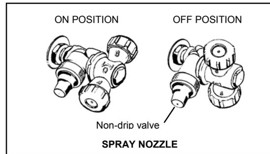
Nozzle direction can be adjusted  $\pm 15^\circ$ . By loosening the attaching nut and angling the nozzle, greater adjustments can be made.
