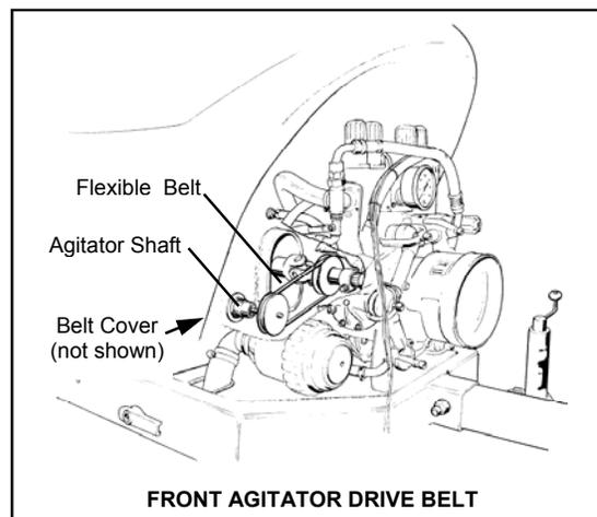
To shorten the belt, remove it from the pulleys and cut it at either side of the join, adjacent to the ends of the connector piece. Shorten the belt to an overall length of 730 mm. Remove the connector from the cut out section and use it to rejoin the shortened belt.
