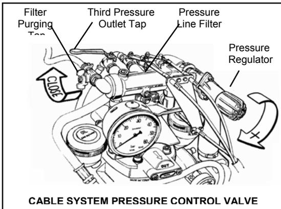
To shut the sprayer down move the central lever to "Off", reduce engine speed and disengage the tractor PTO.
