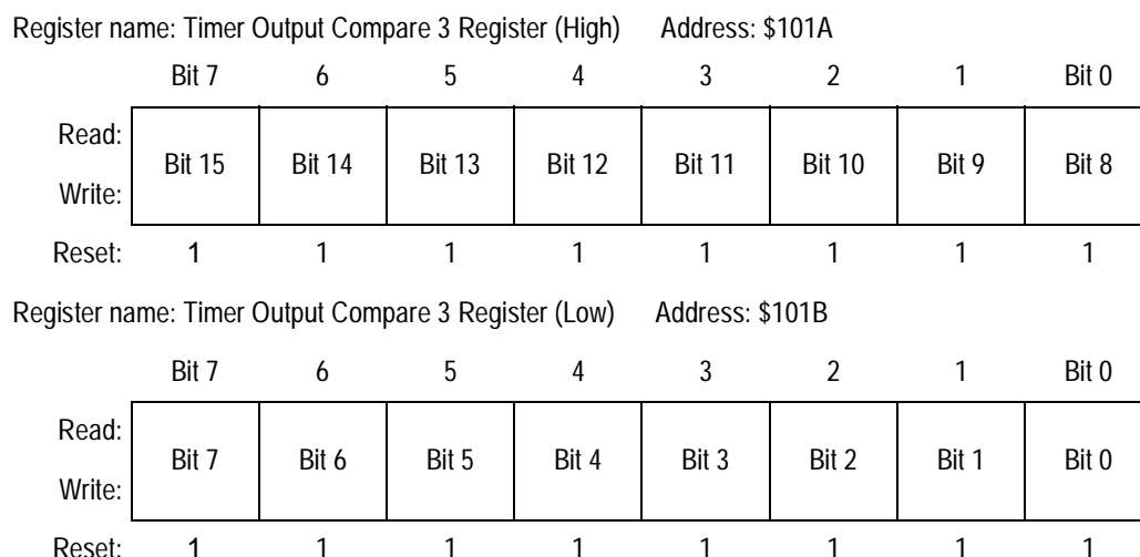
Figure 9-10. Timer Output Compare 3 Register Pair (TOC3)
