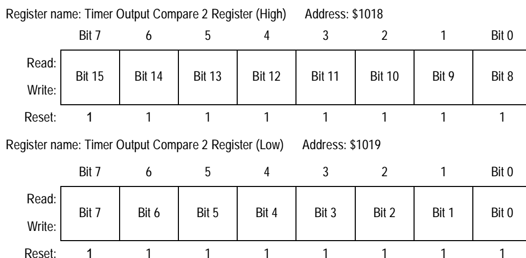
Figure 9-9. Timer Output Compare 2 Register Pair (TOC2)
