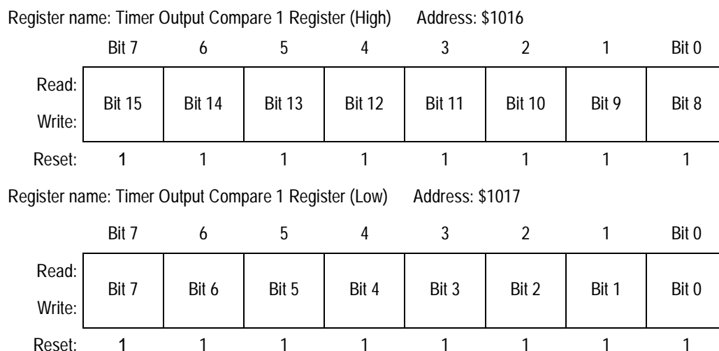
Figure 9-8. Timer Output Compare 1 Register Pair (TOC1)
