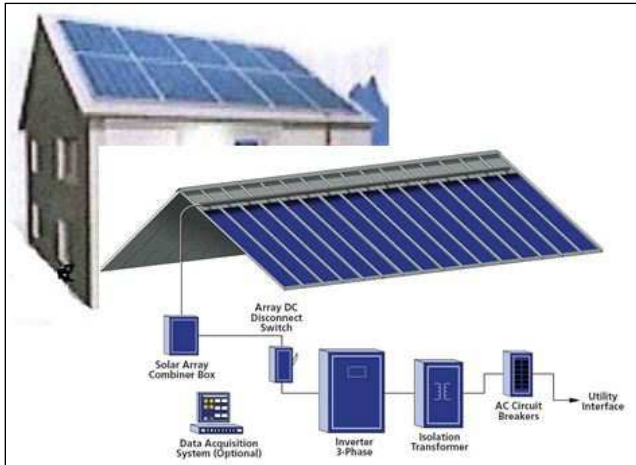
Figure 8-30 Roof Mounted Solar Energy Systems
