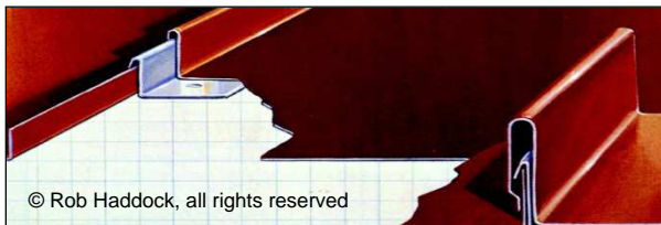
Figure 7-14 Larger Side Ribs Are Used To Conceal Panel Fasteners
