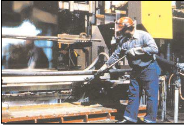
Figure 3-6 Zinc Coating of Steel
