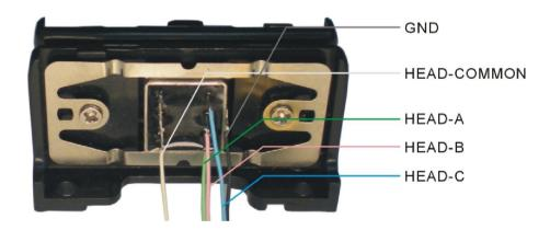
The portable magnetic stripe reader, plastic rail is ideal to test your MCIR001. It includes a 3 track low profile head which can be used to read up to 1,000,000 cards.
