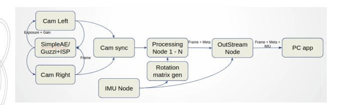
The elements of the diagram above are logical blocks, not necessarily FLIC plugins. The translation of this diagram to FLIC plugin diagram can be found in later sections.
