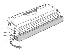
**6** Install the new toner cartridge into the drum unit until it clicks into place.
