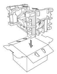
**9** Place documents (manual, printed material and CD-ROM), document tray, and document support, drum unit and toner cartridge assembly, the telephone line cord, power cord and printer cable into the carton as shown below.
