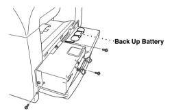
**4** Disconnect the connector of the back up battery.
