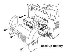
$\mathbf{3}$  Remove the screws securing the access plate and remove the plate.
