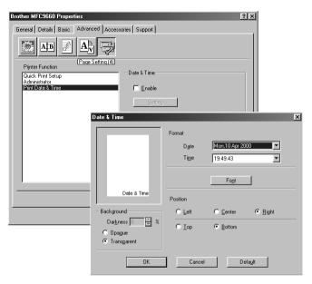
Click the **Setting** button to change the **Date and Time Format**, **Position** and **Font**. To include a background with the Date and Time select **Opaque**. When **Opaque** is selected, you can set the **Darkness** of the Date and Time background by changing the percentage.
