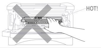
**1** Open the front cover and pull out the drum unit.
