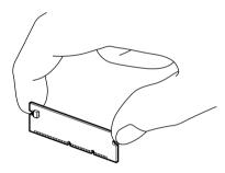
Make sure the memory board is securely seated in the main controller board.
