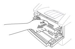
**3** Pull the toner cartridge out of the drum unit assembly while holding down the lock lever with your right hand. (See *Replacing the Toner Cartridge*, page 139)
