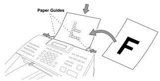
The Automatic Document Feeder can hold up to 30 pages, feeding each one individually through the machine. Use standard (64 gsm~90 gsm) paper when using the Automatic Document Feeder; if you're using heavier paper, feed each sheet individually to prevent paper jams.
