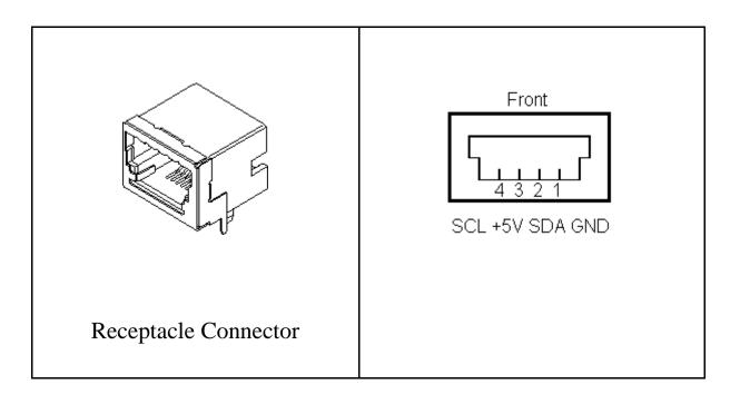
An I<sup>2</sup>C Interface Cable (White=SCL, Red=+5VDC, Green=SDA, Black=Ground) is provided to connect to an external I<sup>2</sup>C Bus. Since there is no standard I<sup>2</sup>C Bus connector, you may want to cut off one end of the cable and add a connector compatible with your target system.
