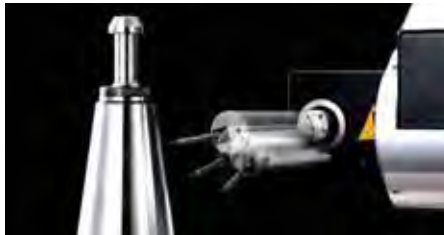
Detector rotation mechanism (0 to 290°, in increments of 1°)
