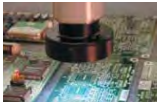
QVP (Quick Vision Probe) For video measurement
