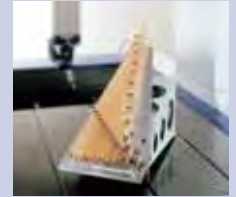
CMM calibration tool using the virtually zero thermal expansion glass gage
