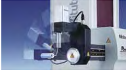
Holder-arm orientation switching (vertical position - horizontal position)
