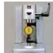
Using test indicator attachment set ( 02ASK000 )
