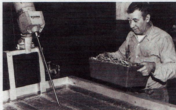
Gear drive portables deliver high flow, high pumping action in wash and treatment tanks for metal parts.
