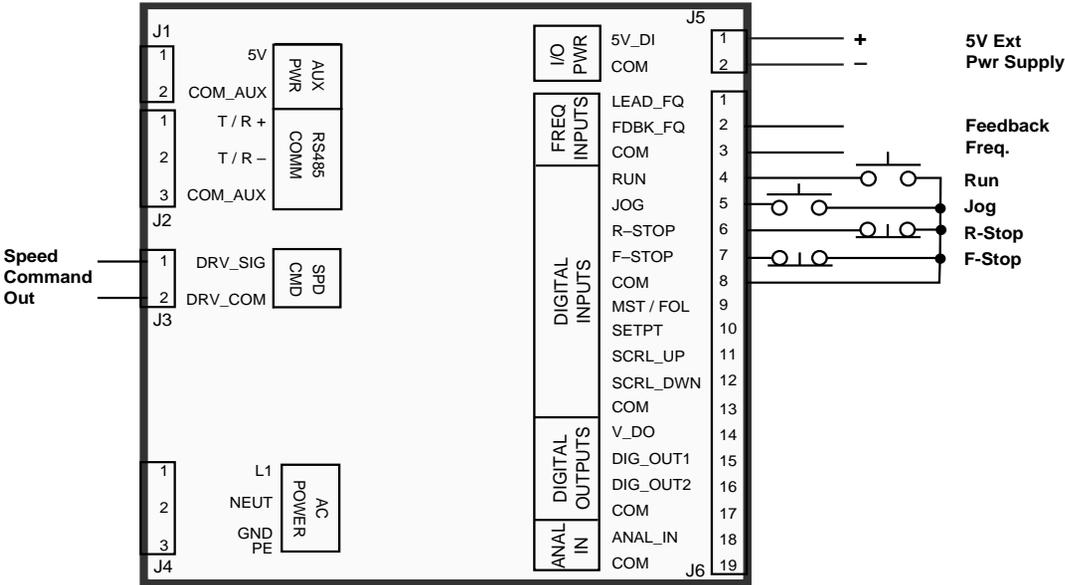
Figure G-1 MLP-Trim Wiring Connections without Relays
