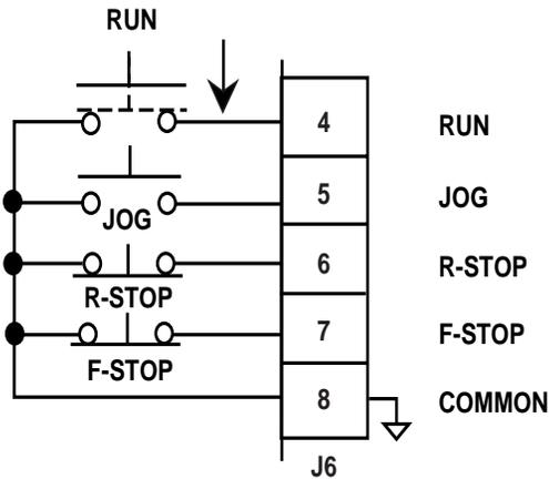
**Jog** has the least operating priority. Jog ramps to the Jog Setpoint (CP-05), using the Acceleration Time (CP-16). When Jog is terminated, the MLP-Trim brings the Speed Command output to an immediate Zero. Unlike the other inputs, Jog is not latched and must be sustained to remain active.
