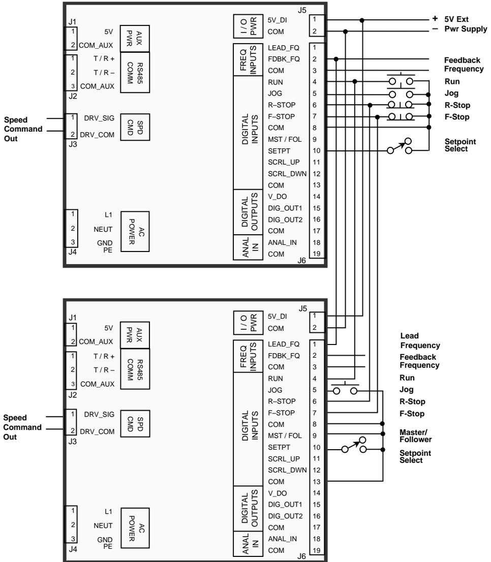
**Figure G-5 Two Channel Start/Stop - Lead/Follower Logic**
