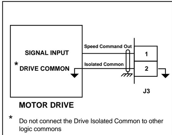
**Figure 2-17 Speed Command Out**
