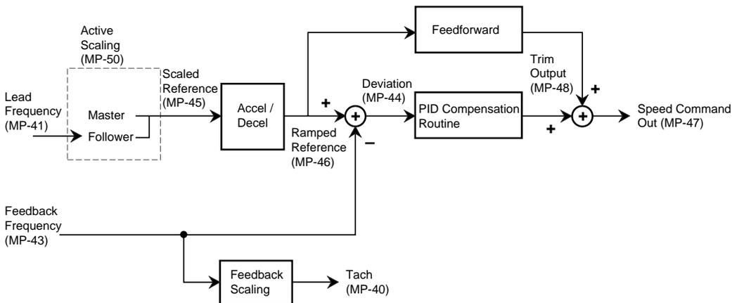
Figure 3-2 MLP–Trim Internal Structure
