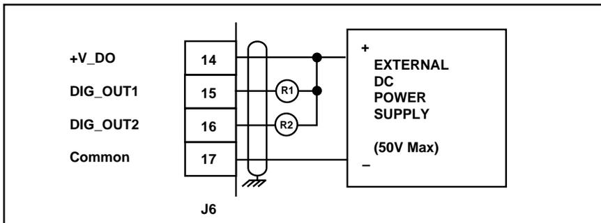
Figure 2-18 Digital Output 1 and Digital Output 2
