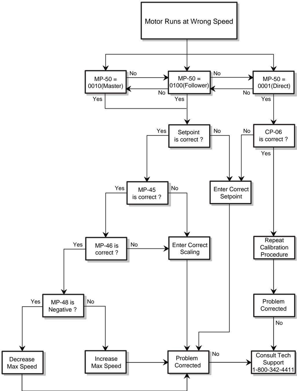
**Figure 4-3 Motor Runs at Wrong Speed Flowchart**
