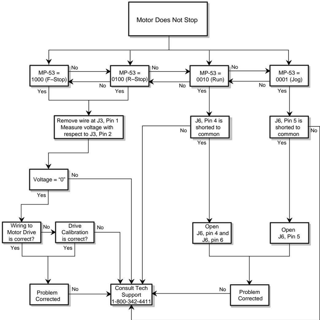
Figure 4-1 Motor Does Not Stop Flowchart
