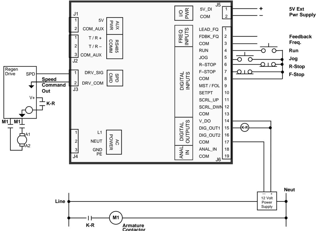
**Figure G-3 Start/Stop for Regen with Armature Contactor**
