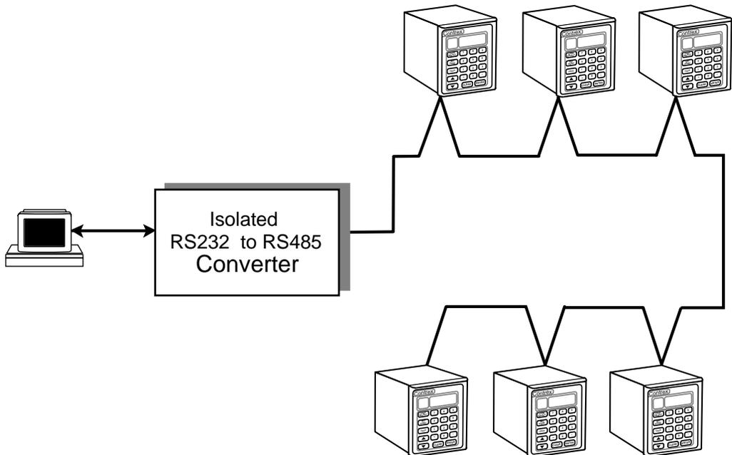
**Figure 2-19 MLP–Trim Multidrop Installation**
