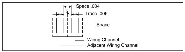
Figure 60. Typical Wiring Channel Top View
