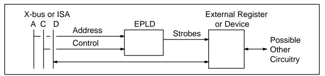
Figure 5. Typical External Register
