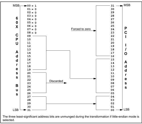
Figure 2. Non-Contiguous PCI I/O Address Transformation
