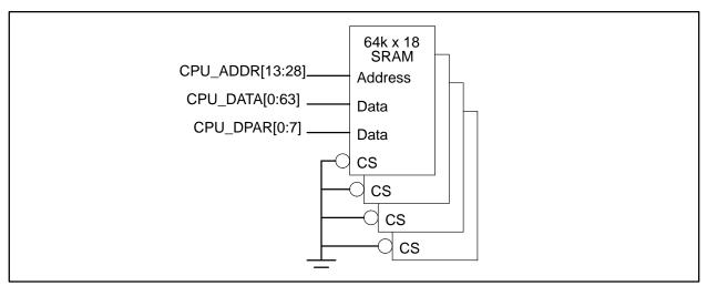
Figure 11. Asynchronous SRAM, 512K L2
