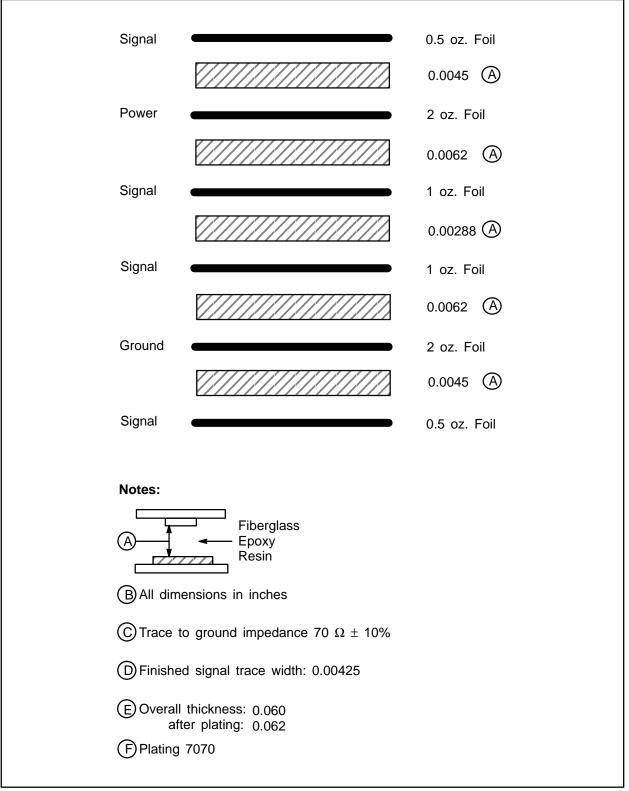
Figure 61. PowerPC 603/604 Board Fabrication
