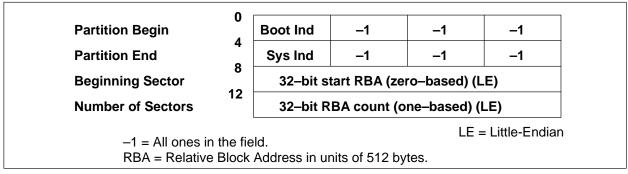
Figure 27. Partition Table Entry Format for an Extended Partition
