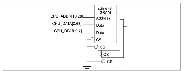
Figure 8. Synchronous SRAM, 512K L2
