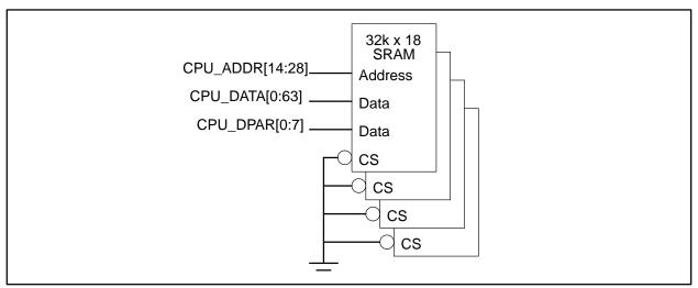
Figure 7. Synchronous SRAM, 256K L2
