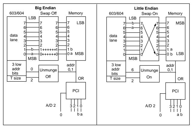
Figure 18. Double Byte Write Data ab at Address XXXX XXX0
