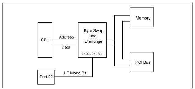
Figure 15. Endian Mode Block Diagram
