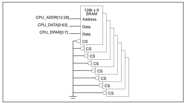
Figure 12. Asynchronous SRAM, 1M L2
