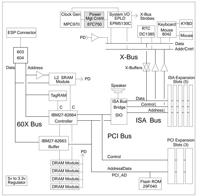
Figure 1. 603/604 Reference Design Block Diagram
