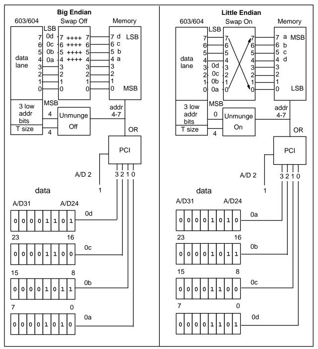
Figure 19. Word (4-Byte) Write of 0a0b0c0dh at Address XXXX XXX4
