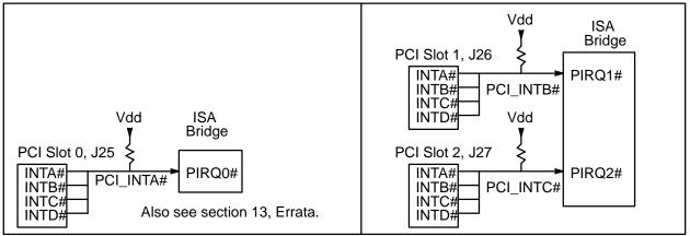
Figure 24. PCI Interrupt Connections
