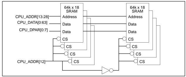
Figure 9. Synchronous SRAM, 1M L2
