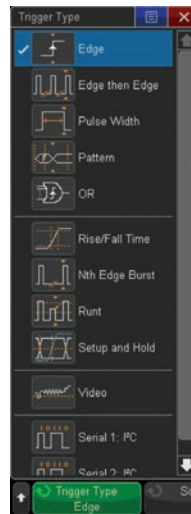
Figure 43. Wide array of advanced parametric trigger modes.
