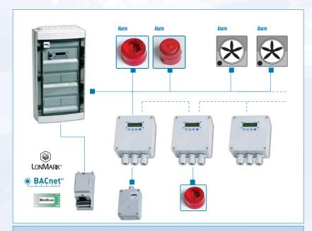
Several single space monitoring systems can be connected to a master controller via bus line. Consequently there is the possibility of a central analysis, central alarms and a connection to a BMS system.
