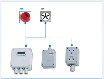
In case of single space monitoring system the leaking gas is measured directly at the SPC (Single-Point-Controller) where also the alarms are given. An external transmitter is additionally connectable. A remote display panel (RDPO3) outside of the danger area for external alarm to avoid entering, is optionally integrable.
