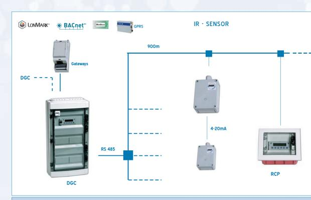
The Controller of a DGC-System manages several sensors via one or more bus lines. Optionally there is the possibility to connect additional analog transmitters to every BUS knot and integrate them into the system.
