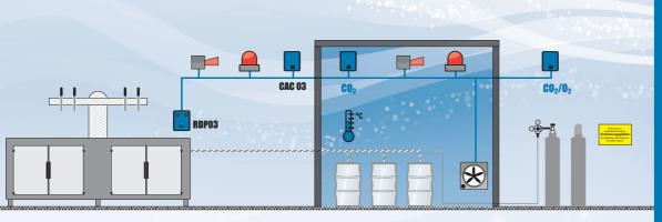
Whether in pubs, restaurants, fermenting cellars, breweries, wineries, bottling plants or even in storage facilities and production halls with  $CO_2$  extinguishing devices, everywhere  $CO_2$  bottles, gas lines and tanks are employed, PolyGard  $CO_2$  /  $O_2$  sensors can be used for monitoring the air quality. Whether for the compliance with the MAC values or for revealing leakages, MSR transmitters always detect reliably harmful concentrations of gases and vapours in the ambient air.
