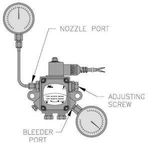
Figure 23: Adjusting Fuel Pump Pressure
