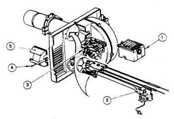
Figure 11A: Installation/Removal of Drawer
