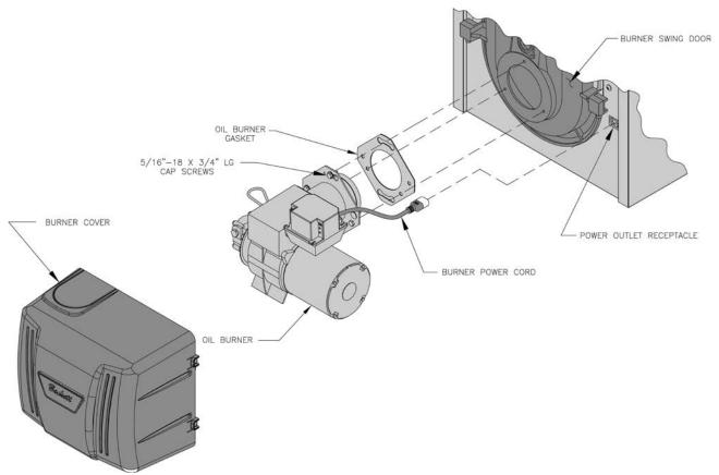
Figure 10: Oil Burner Installation (Beckett Burner Shown)
