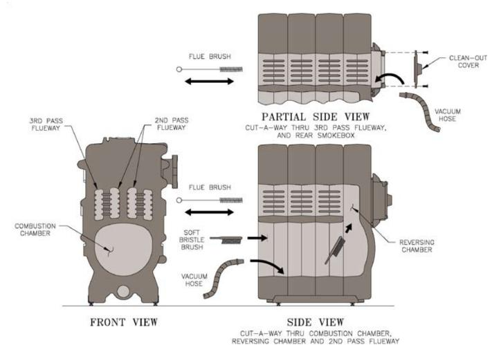
Figure 27: Cleaning Boiler Flueways and Combustion Chamber Surfaces
