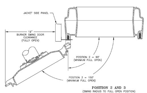
Figure 5B: Top View - Burner Swing Door Mounted to Cast Iron Block Assembly (Jacket Removed for Clarity)
