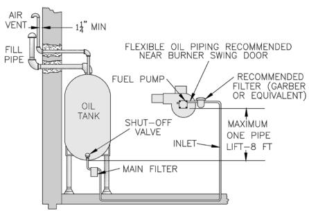
Figure 21: Single Pipe Oil Line
