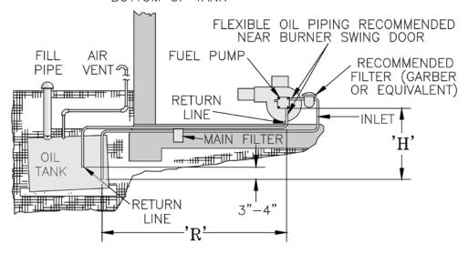
Figure 22: Two Pipe Oil Lines
