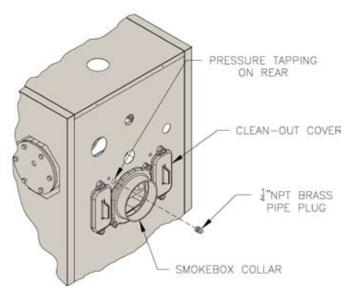
Figure 17: Smokebox Pressure Tapping for Checking Draft at Breech
