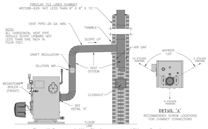
Figure 15: Recommended Vent Pipe Arrangement and Chimney Requirements
