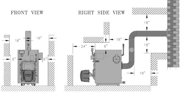
Figure 2: Minimum Installation Clearances To Combustible Materials (Inches)
