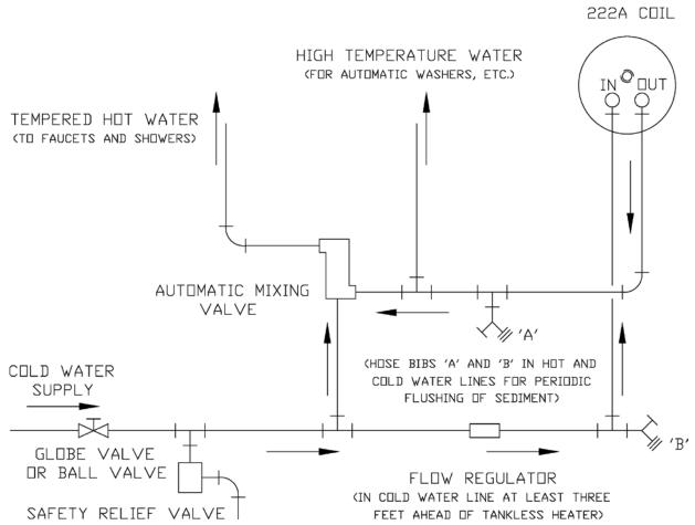
Figure 13: Schematic Tankless Water Heater Piping
