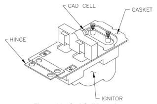
Figure 26: Cad Cell Location
