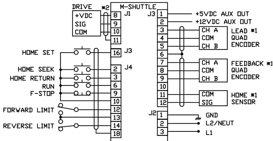
\*1 Encoder and Proximity Switches may require power connections from J3 pins 1 or 2.
