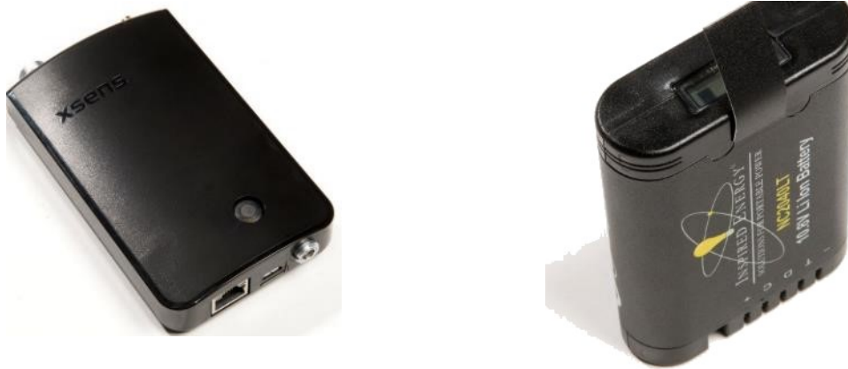
Figure 18: Body pack and battery
