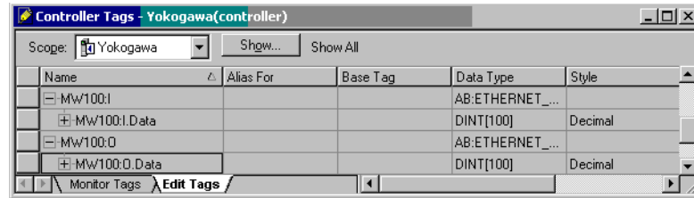
MW100 Channels within RSLogix 5000 Controller Tags Screen
