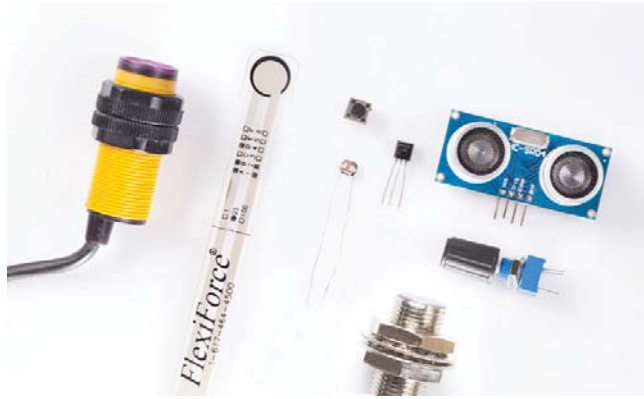
Figure 1-1. Various sensors: infrared proximity, rotation, brightness, button, temperature, and distance
