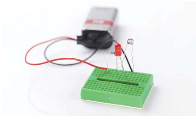
Figure 1-4. The finished photoresistor project
