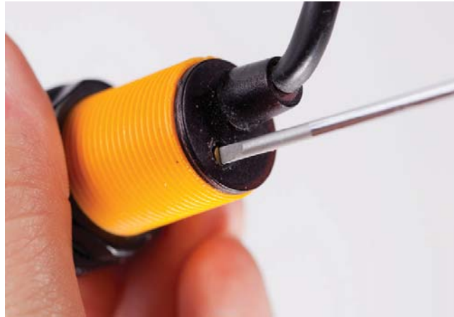
Figure 3-8. Adjusting the infrared sensor
