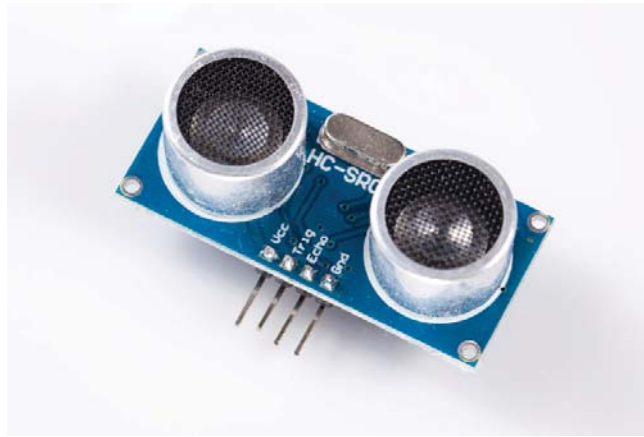
Figure 3-20. Ping ultrasonic distance sensor
