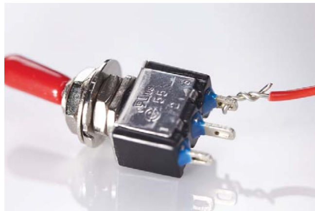
Figure 2-2. Tying a wire to the switch leads
