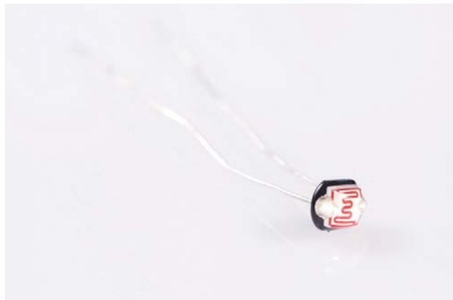
Figure 3-12. A photoresistor is a better conductor in bright light
