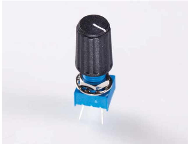
Figure 3-10. Potentiometers can measure rotation
