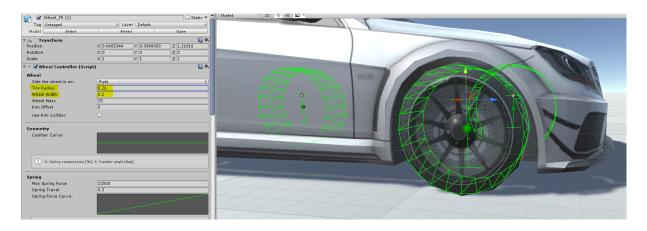
7. Set up **ignore layer**. This is one of the most important steps and if skipped wheels will detect vehicle itself as ground. Create a new layer, name it however you want and assign it to all of the colliders on the vehicle. In this case only the *Body* object has a collider and so it's layer was set to the newly created layer (in this case *WheelControllerIgnore*). You can change which layer you want to ignore at the bottom of the WC3D inspector:
