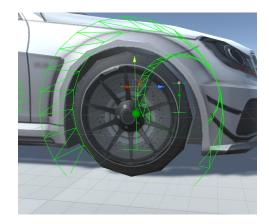
6. Adjust wheel controller radius and width in the WC3D inspector until the green lines fit the wheel.
