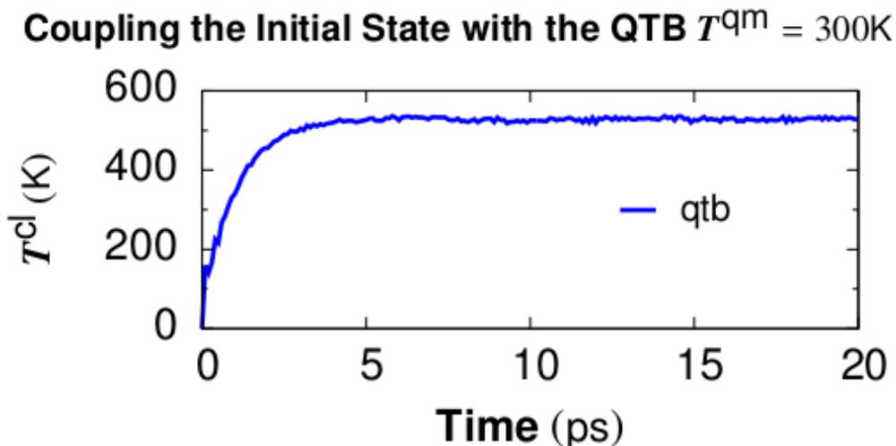
Figure 1. Classical temperature  $T^{\text{cl}} = \sum m_i v_i^2 / 3Nk_B$  vs. time for coupling the alpha quartz initial state with the quantum thermal bath at target quantum temperature  $T^{\text{qm}} = 300$  K. The NpH ensemble is used for time integration while QTB provides the colored random force.  $T^{\text{cl}}$  converges at the timescale of *damp* which is set to be 1 ps.
