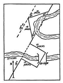
Fig. 10. Two methods of maintaining a compass course around obstacles.
