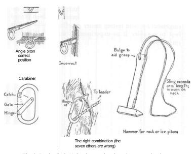
Fig. 3. Rock-climber's hardware, showing piton types in place.
