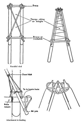
Fig. 16. Parallel and snowplow types of two-ski rescue sleds.
