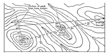
Fig. 11. Method of determining intervisibility.
