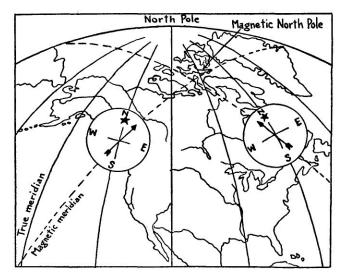
Fig. 9. Relation of magnetic north to true north (simplified).
