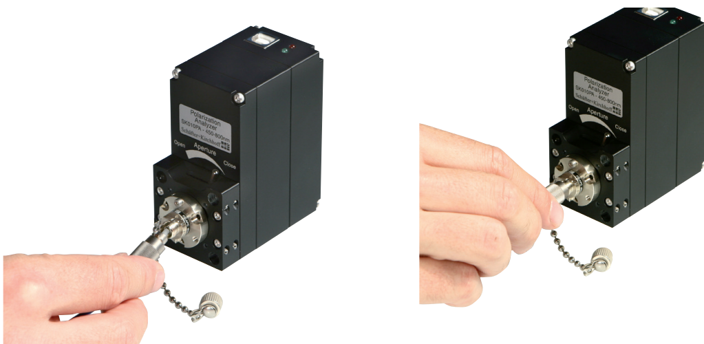
Figure 2: Slopingly attach the connector's ferrule to the fiber adapter in order to avoid damage fits end face. Plug the connector considering its key. Press the connector's key to the right hand side of the adapter's notch. Fasten the box nut handscrewed only.
