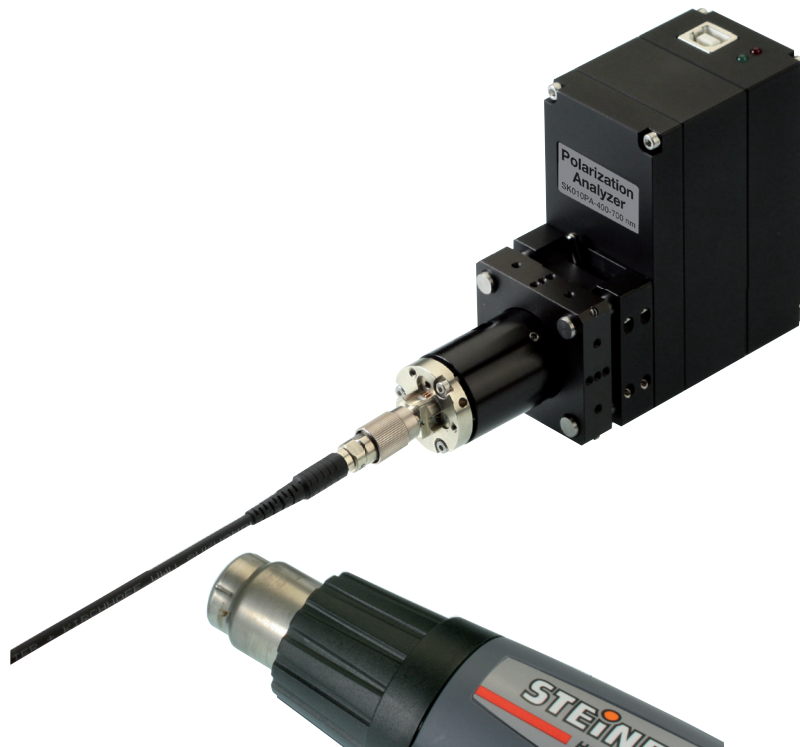
Figure 19: Stressing the fiber thermic with a blow-dryer
