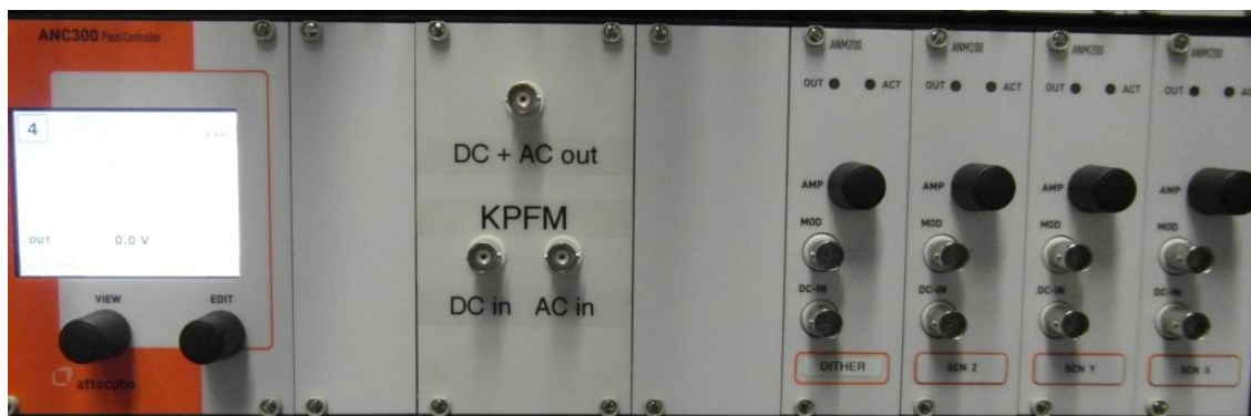
Figure 7: ANC300 used as high voltage amplifier on the axes 1-4, and as a AC-DC coupler for the tip voltage.
