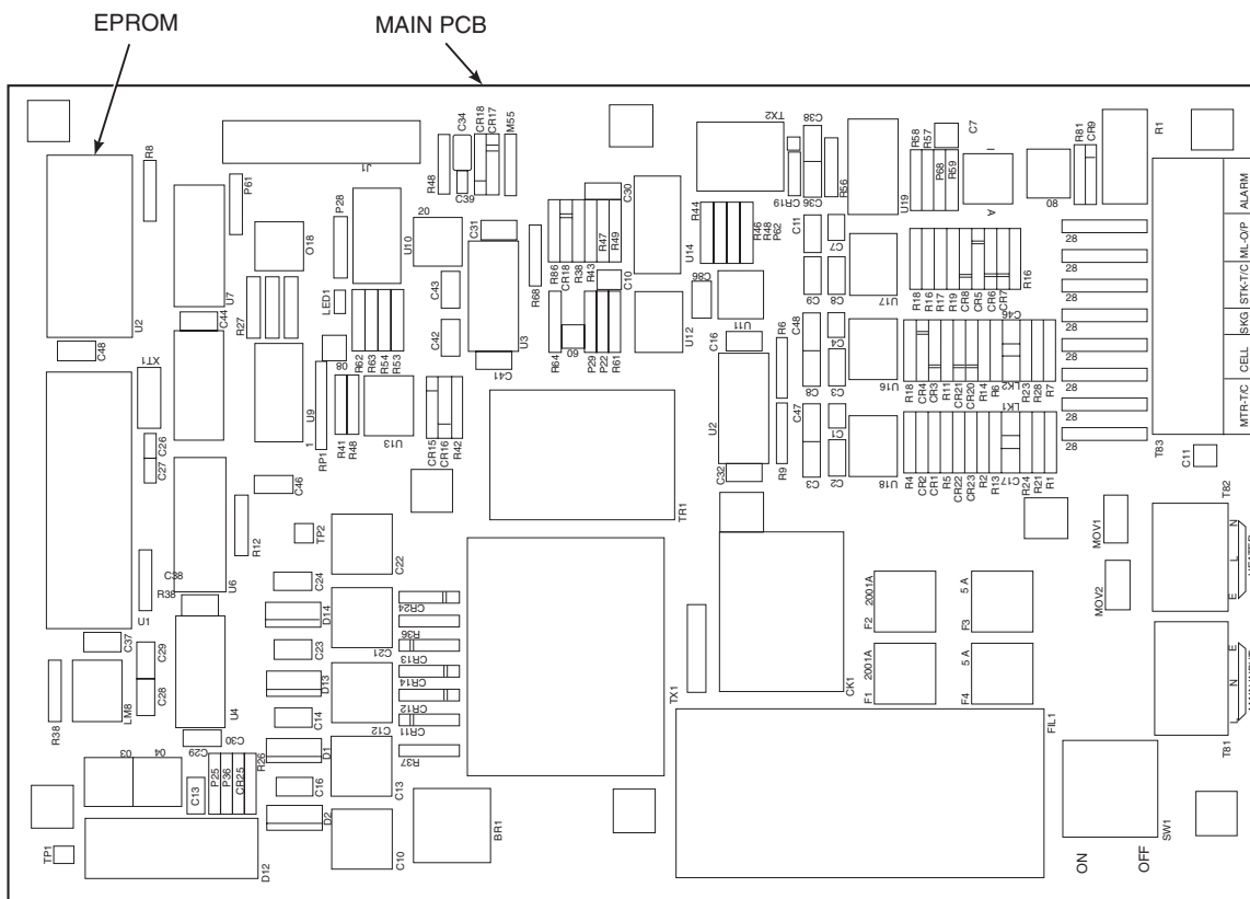
Figure 2-13. Main PCB (Model 132) EPROM Replacement
