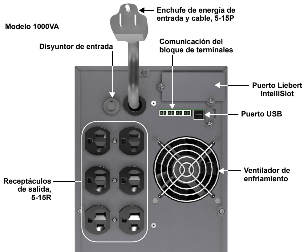
Figura 5 Liebert GXT3-1000MT120™—componentes del panel trasero
