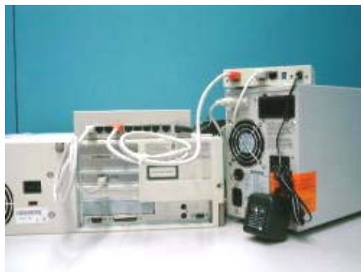
Figure 2-20 Connecting the Ethernet cable from the LAN port of USHA ProE II.
