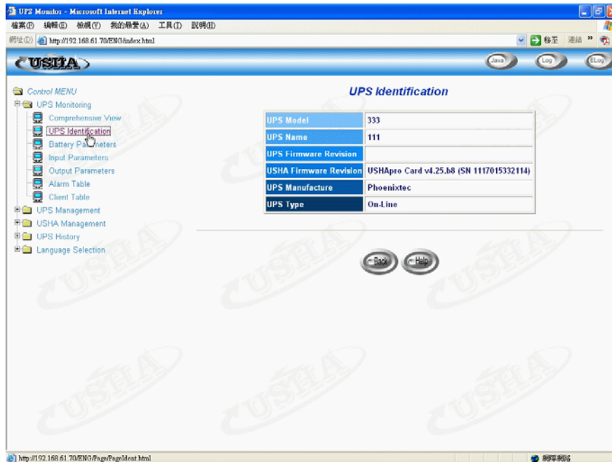
Figure 3-2 USHA UPS Monitoring page screen: UPS Identification.
