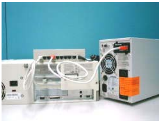
Figure 2-19 Connecting the Ethernet cable from the LAN port of USHA Card.
