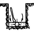
4. Tamp soil between pipeline and trench wall at both sides.
