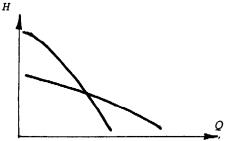
The head H as shown in the characteristic curves of centrifugal pumps is the total or <u>manometric head</u>, i.e. the increase in pressure that takes place between the suction and discharge branches of the pump, expressed in meters liquid column.
